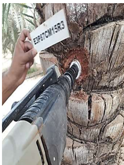
Figure 1. Drilling and sampling procedure for trunk samples.
